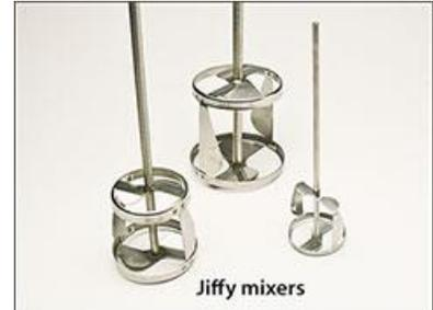
Use a stainless steel spatula or hand-held power mixer to agitate. A paint mixer blade or mortar mixer blade (such as Jiffy Mixers) attached to a power drill is recommended for the mixing a larger amount. Scrape the side and bottom of the mixing container with a spatula as you agitate with a power mixer to ensure homogeneous mix.
