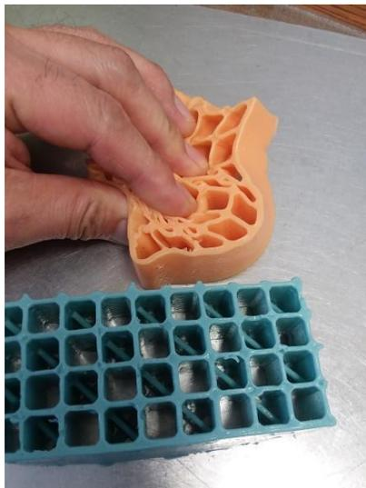
Unlike TPE, MGP-V30A is a thermosetting material that can be processed at room temperature with ambient pressure. Inexpensive soft molds or plastic/resin molds can be used to mold parts of this material. For small production quantities, it can be processed manually without a specific processing/dispensing machine. These easier processing parameters make MGP-V30A an easier and low-cost alternative to TPE.
