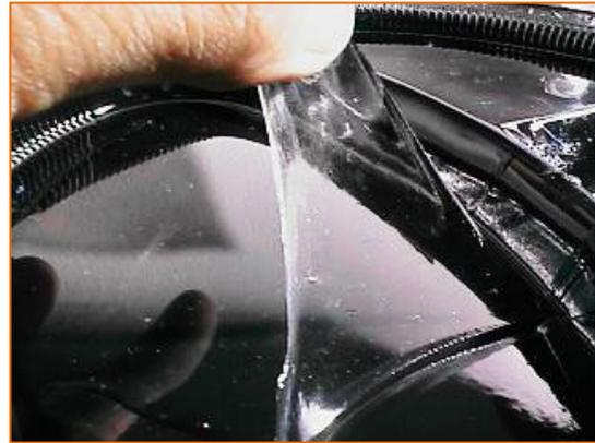
Unlike other PSA tape products, GK-7R4 can be made to have a sticky surface that does not leave residue on substrate surface. The stickiness can be adjusted by simply adjusting the mixing ratio between the given part-A/part-B components so that the processors can fine-tune the stickiness of their products without formula modification.
