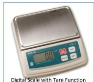
Put a mixing container on a scale. Using a digital scale with Digital Scale with Tare Function tare function is recommended. The mixing container should be a clean/dry disposable round container with a smooth flat bottom. Plastic pails, tin paint cans, and plastic cups are some of the recommended containers.
