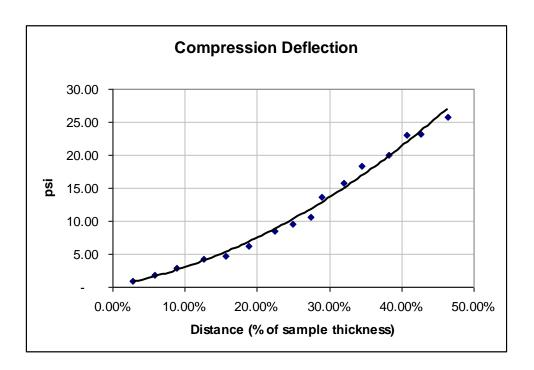
The above data is typical properties of the free-risen foam tested in our generic test method. Compression-molded foam will have different deflection property.
